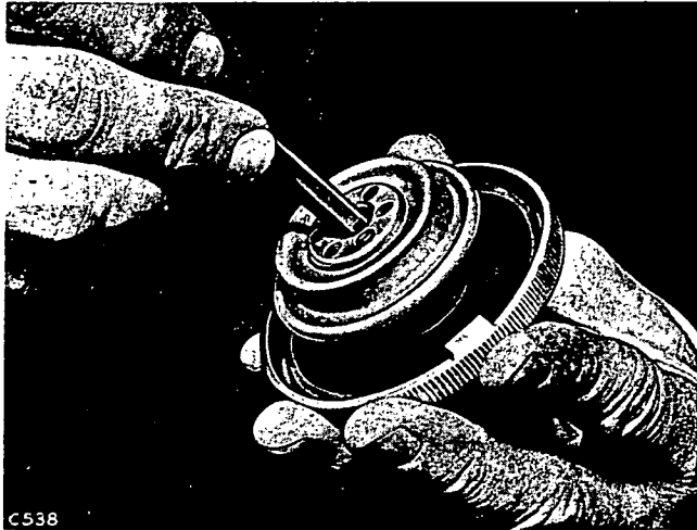
Fig 96. Checking radiator pressure release and overflow valve
